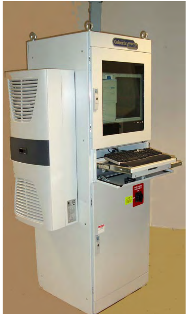
NEMA 12 Plant Floor Control Unit
